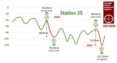
At Station 25, 48.6mm of subsidence was recorded from May to October in 2018, and 52.9mm between April to August in 2022. Movement in the intermediate years was 42.3mm in 2019, 30.5mm in 2020 and 8.3mm in 2021, reflecting the problems associated with predicting the risk of root induced clay shrinkage. The interval between readings varies by year and the above are approximations only.
