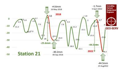
At Station 21, above, 30.2mm of subsidence was recorded in 2018 between May and September (readings are generally taken at two-month intervals), and 44.5mm between April and August 2022. 2019 and 2020 have similar values.
