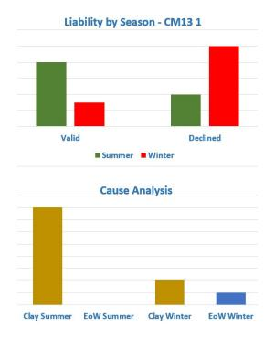
**CM13 3** – A similar profile to CM13 1 above, with clay shrinkage being the most likely cause of damage in the summer months, and a high probability that a claim is likely to be declined in the winter.
